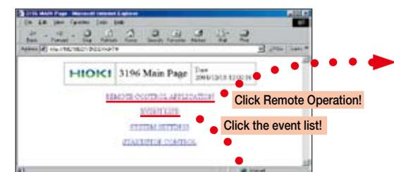
2. A display screen and operation keys identical to those for the 3196 appear, allowing full control of remote operation.
